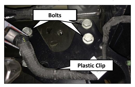
Install the bumper step by lining up the holes of the bumper step with the holes in the truck. Then reinstall the factory bolts that were removed in step one. Ensure that the wiring is not in the way and Fully tighten the hardware.
